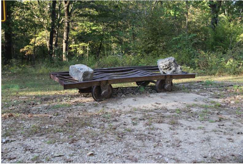
Figure 2-5. A rail cart used in transporprting quarried Gunter Sandstone during construction of the Castle.
